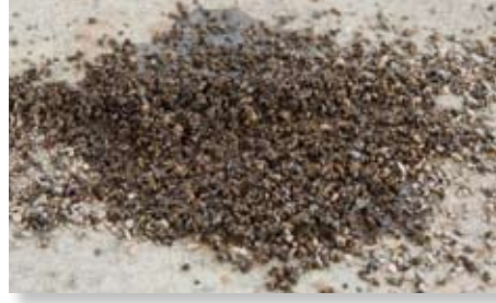
Oil is smeared over the floor surface as clay comes in contact with the spill.
