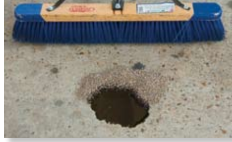
Clay applied to a spill
